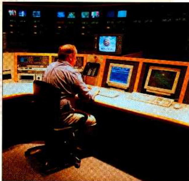
The transmission control room at Speer Communications, Nashville, features the Alamar Media Manager, the DEC Alphastudio terminal, control terminals for two Philips Media Pool video servers and TDC undermonitor displays.
