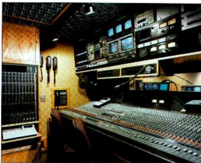
The main audio mix position of the NDTC remote truck places processing gear, recorders and communications all within easy reach.
